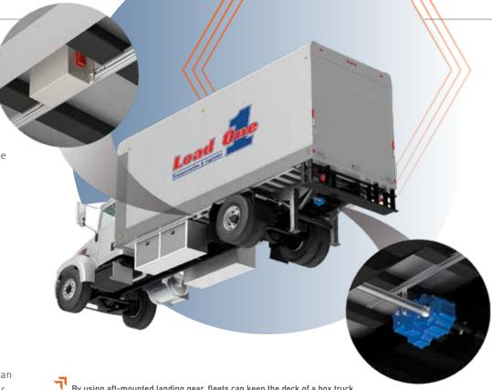
By using aft-mounted landing gear, fleets can keep the deck of a box truck stable and flush with the dock during loading operations using heavy forklifts.
